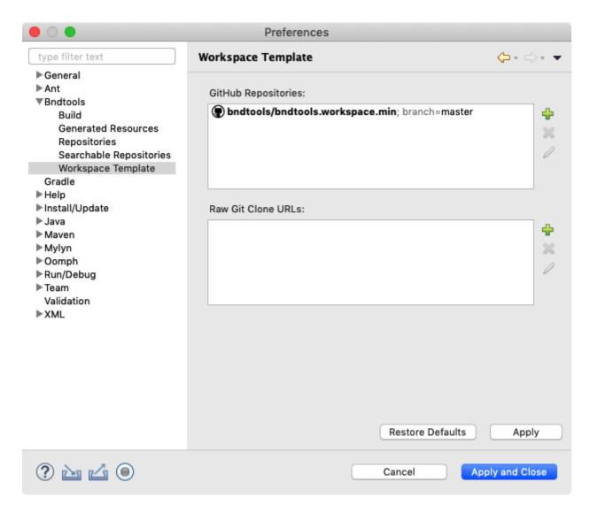
Ensure that the *template* bndtools/bndtools.workspace.min is in this list for the master branch. Press the **[Validate]** button to verify that you entered this template's address correctly. You can find the content of this workspace template here:
