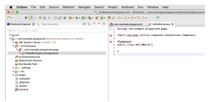
The source contains errors because we have not yet added any dependencies. Since the source uses the OSGi component annotations, the compiler cannot compile the source code. You can use the quick fix (The little yellow light bulb with the red cross) to add the OSGi annotations as a dependency.
